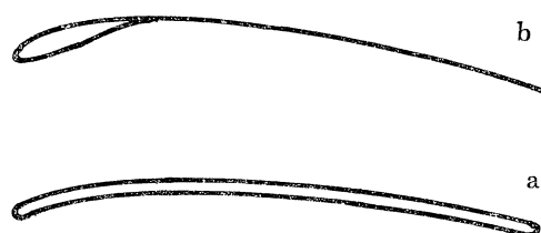
FIGURE 43. Wing sections. (a) Gottingen 417a; (b) Pteranodon ingens .
